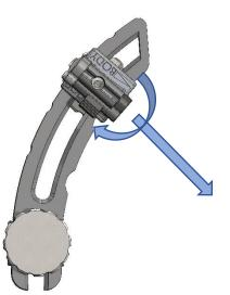
NOTE: To ensure correct assembly for left or right knee configuration, make sure that the word "BODY" (highlighted below) on the Trocar Guide Base is readable in the shown orientation and that the arrow points towards the patient. The direction of rotation of the swivel lock changes based on the left/right orientation.
